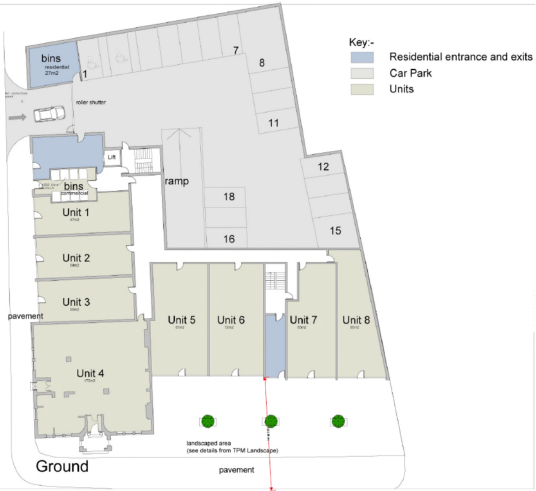
Proposed ground floor layout plan
